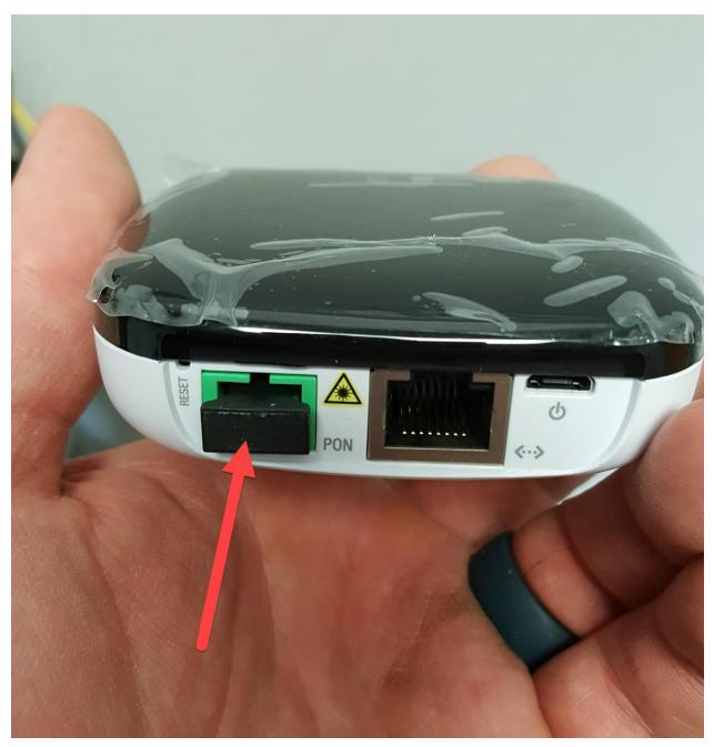
There is notch on the fiber cable port so it will only go in one way, **do not force it**. You should hear a click sound when it is seated in.
