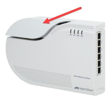
That cover can be removed by pulling it directly away from the backplate. This may require a little force.
